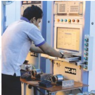
Surge Impedance Test
