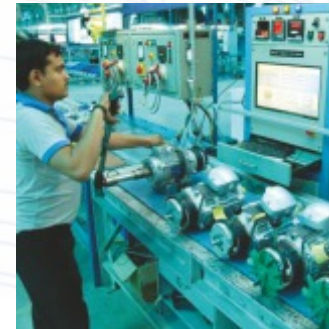
Brake Motor Testing
